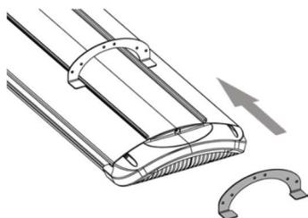
**3.** Insert the arch- shaped support in the special rail on the upper side of the device
