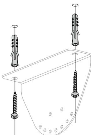
2. Fix the two supports to the wall using dowels of appropriate size.
