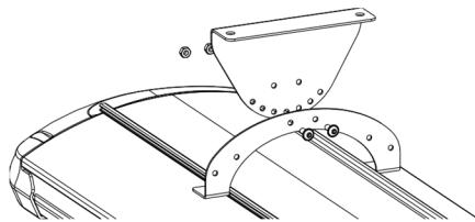
The support to be fixed to the wall presents a series of holes that allow to fix the heater in different positions.
