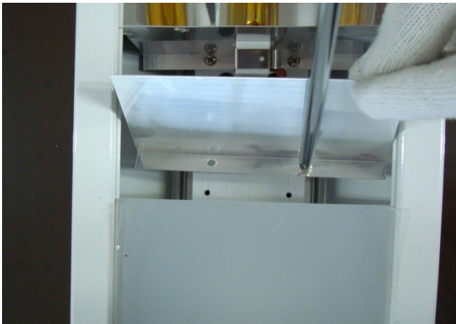
Step 8_Loosen Screws in end plate remove the plate in the info field
